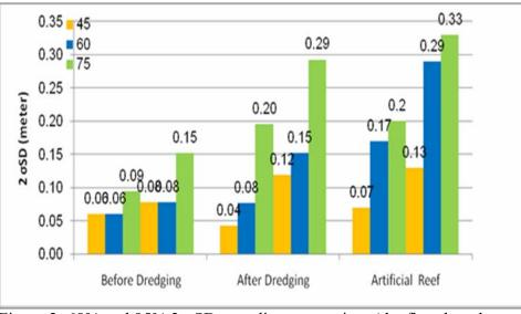
Figure 2: 68% and 95%  $2\sigma$  SD sounding uncertainty (the first three bars from the right in each project are 68% and the second three bars: 95%)
