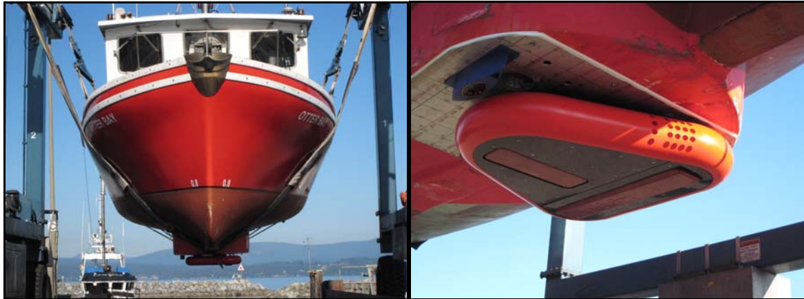
Figure 4 - Otter Bay (left); pod modifications/adaptor plate/EM2040 (right)
