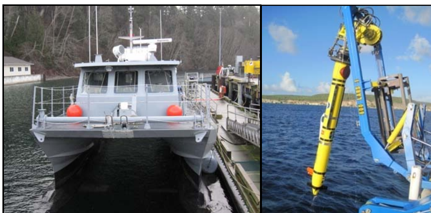
Figure 3 - SWATH boat (left) and REMUS AUV with EM3002 being deployed (right)
