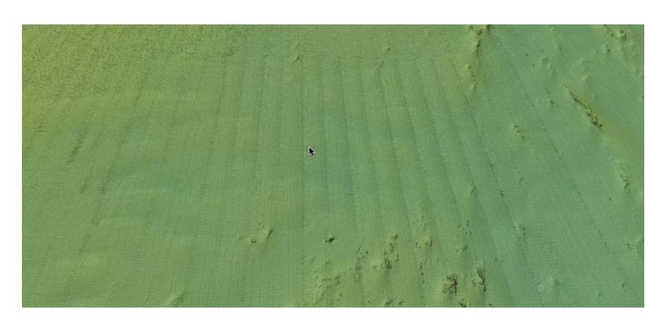
7125 Data Reduced with a single point correction - Differences of between 10-20cm between lines
