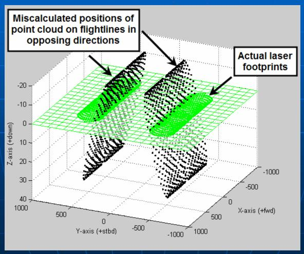
Even heading boresight misalignments can be determined from a flat featureless surface – provided the vessel surveys with ~attitude~ (not altitudes)
