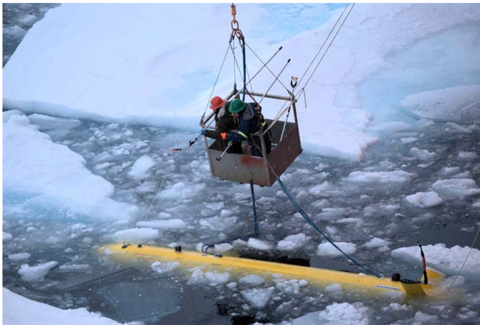
Figure 10 Recovering the AUV in Arctic waters
