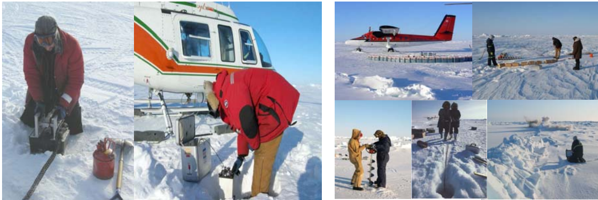
Figure 4 Collecting bathymetry and gravity to determine the shape of the seafloor
