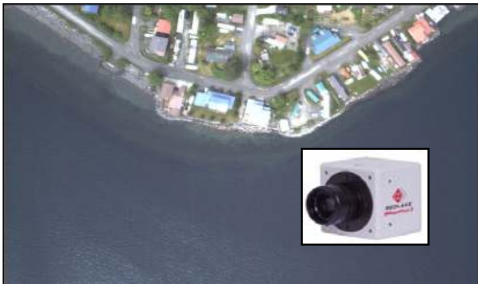
Figure 2: An example of imagery captured during survey operations around Craig, AK. Inset: The Redlake MegaPlus II ES 2020 digital camera
