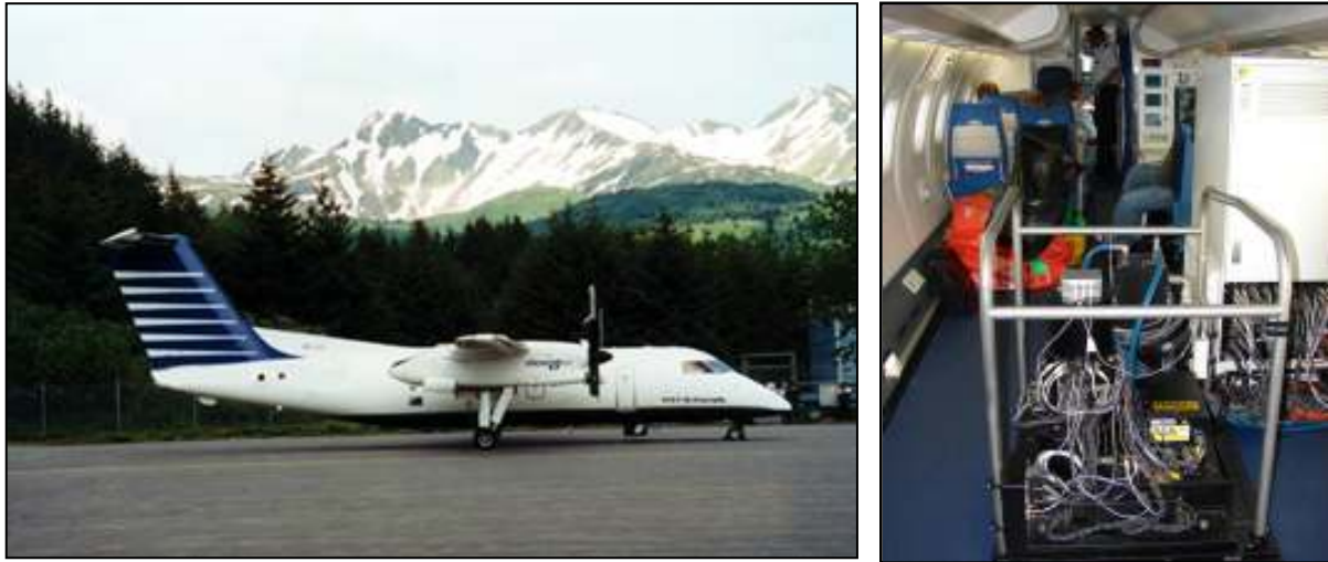
Figure 1a: Tenix LADS deHavilland Dash 8 200 Series bathymetric lidar survey platform. 1b: LADS MkII lidar system
