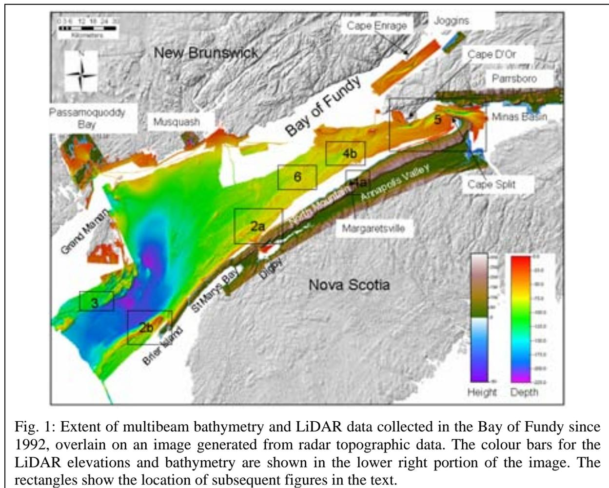
Fig. 1: Extent of multibeam bathymetry and LiDAR data collected in the Bay of Fundy since 1992, overlain on an image generated from radar topographic data. The colour bars for the LiDAR elevations and bathymetry are shown in the lower right portion of the image. The rectangles show the location of subsequent figures in the text.
