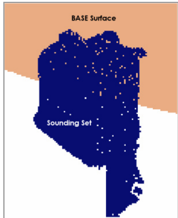
Figure 6 - Contribution layer of a Product Dataset generated from a BASE Surface and a Sounding Set when the dataset level attribution selects the Sounding Set. Spatial extent is 925m x 1140m gridded at 8m.
