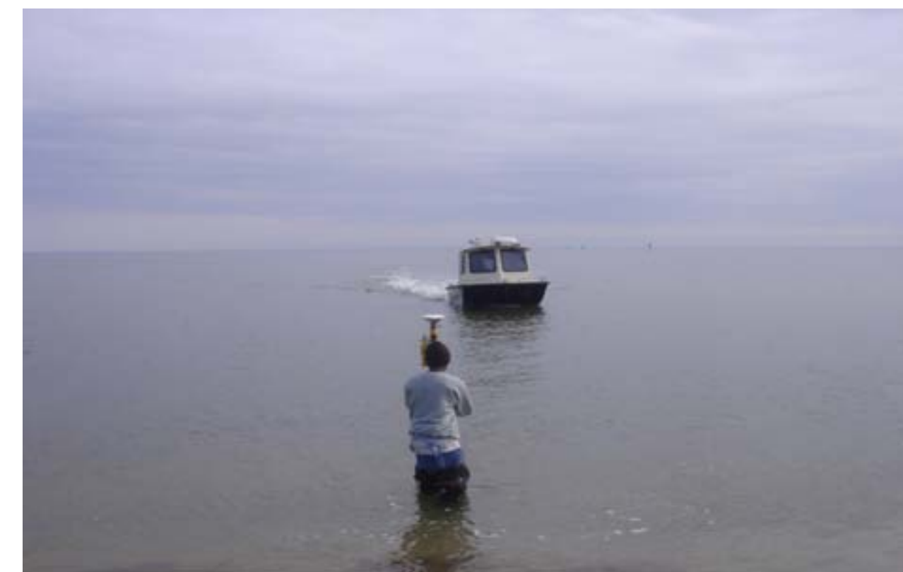
The boat coming in on a cross-section meeting up with the Topo Topo: Trimble RTK 5700 unit Hydro: HYPACK software for the Hydro GDPS and Odom CV3 Depth Recorder on board
