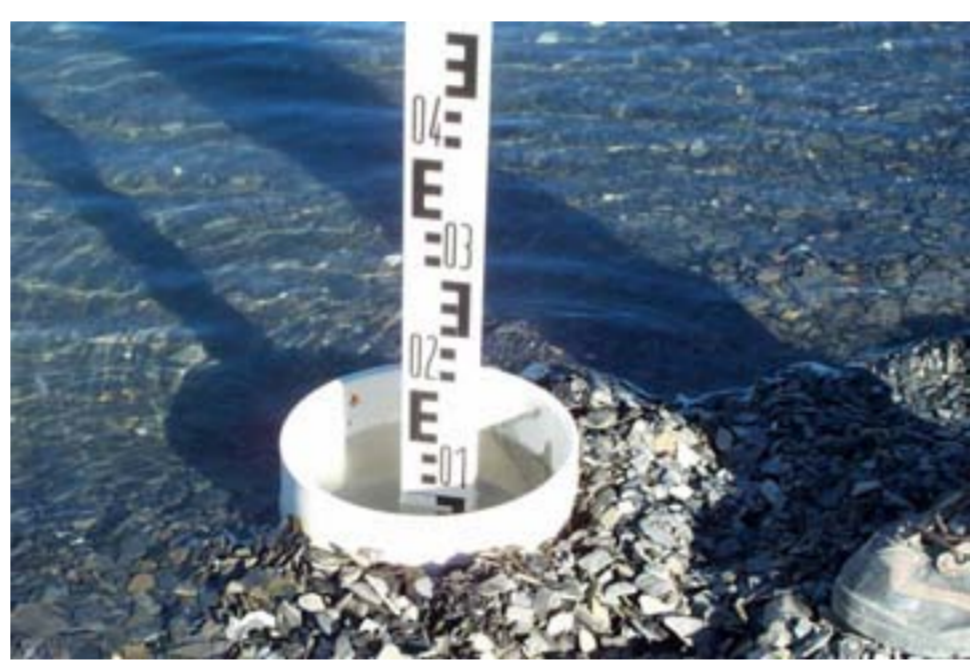
Figure 8. Stilling well / gnomon set-up at Alert.
