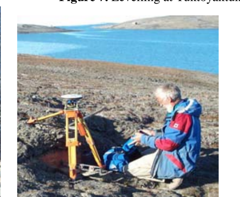
Figure 9. GPS Observations on a bench mark at Alert.
