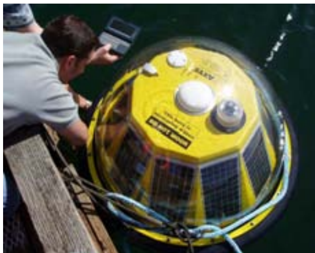
Figure 6. The 0.9-meter buoy with Tri-band Antenna (GPS L1/L2 and INMARSAT L-band) and solar panels.
