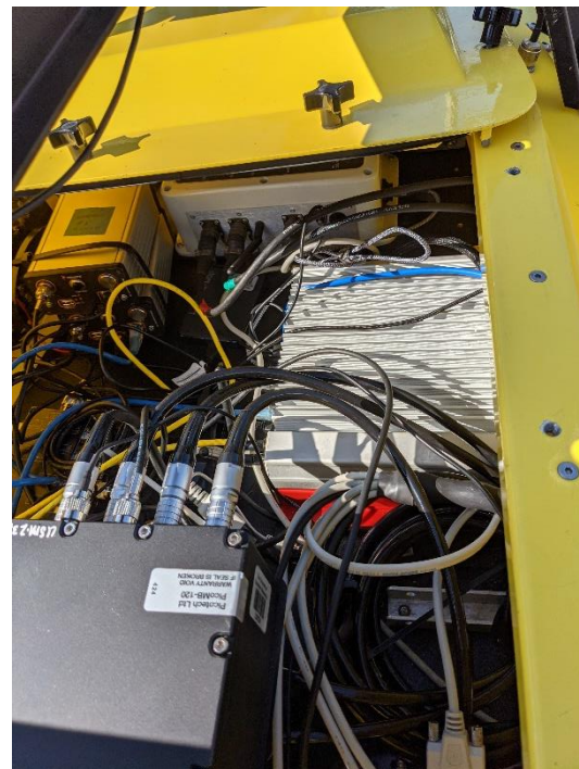
Echo boat's payload contains hardware setups involving two units of Septentrio Mosaic receiver, 1 Droteck (Ublox F9P), and an Applanix survey-grade GNSS+INS
