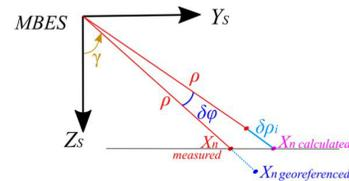
Fig. 1. Pointing error (cyan). When:  $X_n$  is the surveyed point,  $\rho$  is the distance measured between MBES and the seabed,  $\gamma$  is the angle between the nadir and the beam direction and  $\delta\varphi$  the uncertainty in the roll angle.
